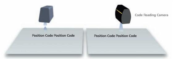
The flexibility of Cognex's patented line synchronization technology enables additional code marks to be added if the original codes are trimmed off or coated over. Additionally, the codes may also be configured to include unit identification numbers in order to ensure accurate product tracking. The accuracy of the position code
